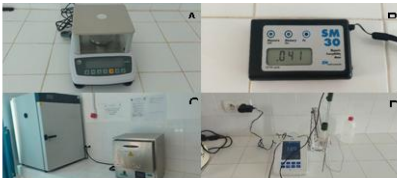
Figure 4: Laboratory equipment employed for the examination of the soil properties attributes of Boudinar soil samples includes: A: analytical balance B: susceptibility meter, C: drying furnaces, D: pH meter
